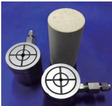
图 3 渗流专用压头 Fig. 3 Special indenter for seepage
